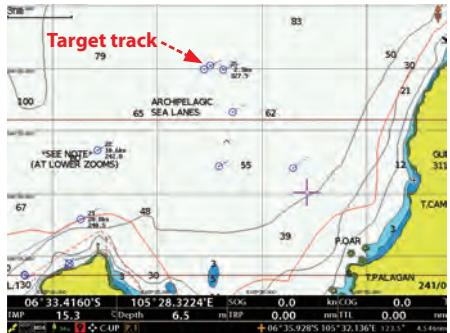
The radar's TT functionality displays the trails of other ships.
